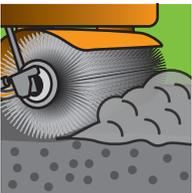
Make sure the surface to be tacked is thoroughly clean and free of dust and debris prior to application of CleanTac. Note: product can adhere to dust and debris and thus peel off surface when dump truck traffic is present.
