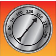
Initial heating of CleanTac is 150°F while circulating only if temperature at time of application is below 140°F – If not only circulate. Heat tubes must be covered to achieve heating. Note: To calibrate distributor thermometer please periodically check temp of actual material from spray bar and compare, notating degree difference.
